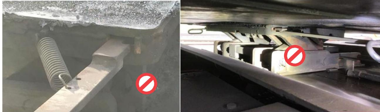
**Note 7: Visually check that the semitrailer is loaded correctly and the kingpin is in the right position inserted into the guide ring**
