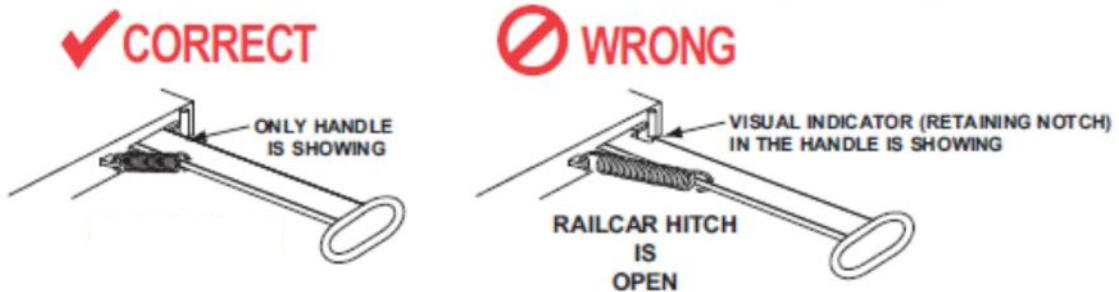
**Pictures of a modified handle in open position.**
